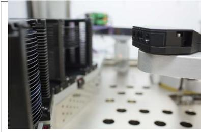
Laser sensor slot-scanning to check wafer size, carrier type, double- or cross-loaded slots.
